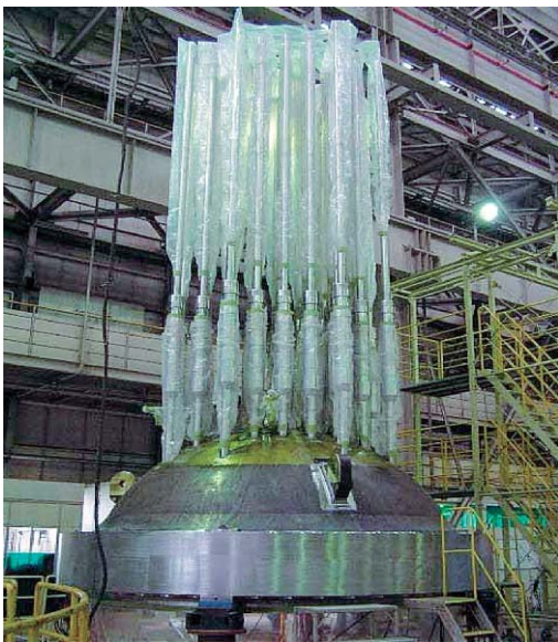
Fig. 4 Reactor vessel closure heads and CRDM Reactor vessel closure heads and CRDM assembled in factory. Base nozzles of CRDM are shrunk-fit, assembled in reactor vessel closure heads, and joined by J-groove welding.
