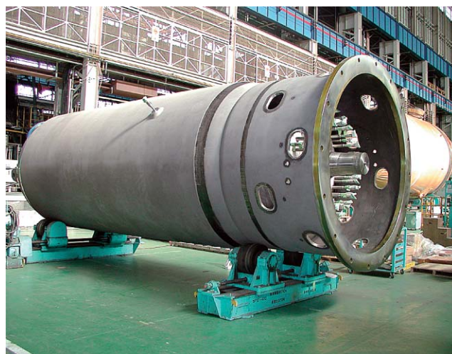
Fig. 6 Replacement Pressurizer Completed state of replacement pressurizer.
